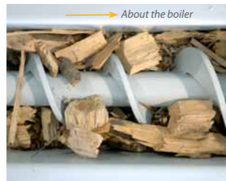
The progressively larger spiral of the worm shaft ensures the uniform and fault-free delivery of fuel.
