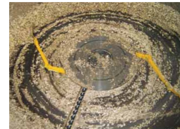
With larger diameters of up to 5.7 metres, the HDG hinged arm delivery system can be used. Even large bunkers with great filling heights (7 metres with a bulk weight of 250 kg/m 3 ) can be reliably emptied by the two pre-tensioned arm elements.
