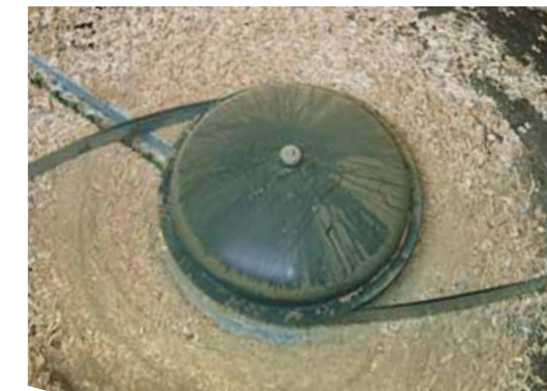
The HDG flexi-blade delivery system is the most commonly installed HDG delivery system. It is suitable for bunkers with a diameter of 2.5 to 4.5 metres.
